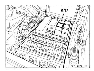
Under these conditions the electromagnetic clutch of the air pump is switched on by the control unit CIS-E (N3) via the relay (K17, see electrical wiring diagram). Via the same relay, the change-over valve (Y32) is actuated at the same time which in turn releases the vacuum to the air shut-off valve (126).
