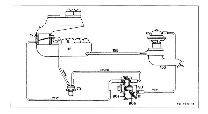
Function diagram exhaust gas recirculation with vacuum control valve up to 08/87
