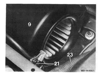
5 Unscrew two screws on temperature switch (21) and pull temperature switch out of blower housing.
