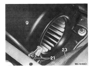
9 Mount electric flat plug and check temperature switch (21) with heating water pump for operation.
