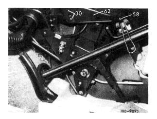
11 Screw oval head screws (57) to tank filler neck.
