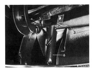
Attach second, longer torsion bar 5.5 mm thick first to hinge lever for top well lid (6). Tension spring by 1/2 turn and attach to trunk lid hinge (5).
