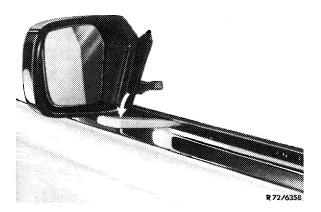
**3** Push lock washer (1) out of handle (2) in direction of arrow.
