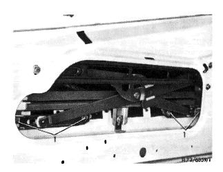
**5** Loosen window guide front (2) on lower fastening (3) and upper fastening (4).
