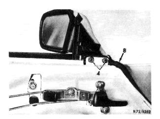
**6** Loosen upper fastening (5) and lower fastening on window guide rear.
