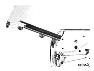
3 Tilt crank window and remove with care.
