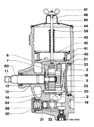
22 Screw guide sleeve from 116 589 24 33 00 (050) on drive shaft.
