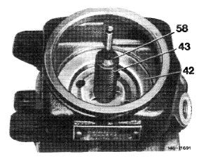
19 If a new volume control valve is installed, make sure that the pressure relief valve has the correct opening pressure. Also pay attention to manufacturer of volume control valve.
