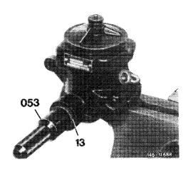
8 Place pressure plate (14) at drive end with groove (arrow) in upward direction over setpin into housing.
