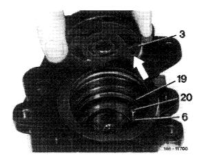
13 Insert O-ring (21) into housing, place compression spring (5) on pressure plate.
