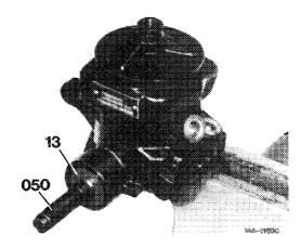
7 Press radial sealing ring (13) into housing by means of pressing-in mandrel. Insert Woodruff key into groove of drive shaft.
