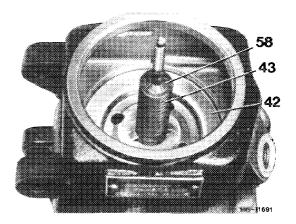
13 On light alloy power steering pump 1st version, place steadying basket (60) into housing.
