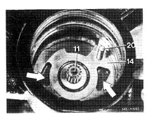
9 Insert cam ring (6) with direction of rotation arrow (arrow) in upward direction into housing.
