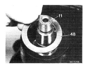
6 Screw guide sleeve from 116 589 24 33 00 (050) on drive shaft.
