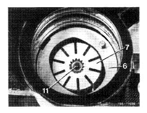
11 Insert blade (16) into grooves of rotor in such a manner that the rounded off sides are facing outwards toward cam ring.
