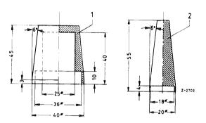
Note: The service-free joints are filled with grease for life. On these joints, sealing against penetration of dirt is of decisive inportance for life of joint. For this reason, a damaged rubber boot must be replaced immediately, since otherwise the entering dirt will result in worn joints. For the same reason, it is also necessary to check the joints regularly and carefully.
