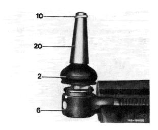
8 Place assembly bushing (21) on ball joint and over rubber bushing (2) and insert flat wire clamping ring (3).
