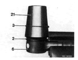
Note: Assembly bushings are self-made according to specified dimensions.
