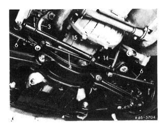
2 Remove track rod (6) on steering arms with puller (25).
