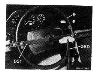
5 Readjust steering if, while turning steering from lock to lock, there is no more increase of friction value in center range.
