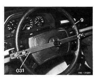
4 Place torque wrench (060) into mounting (031) and turn steering several times from lock to lock. Measure friction torque while turning steering wheel.
