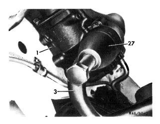
3 Fasten mounting for torque wrench to steering wheel.
