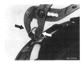
Attach four holding springs to cover spaced 90° apart.
