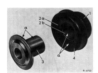
Rubber slide bearing (DU bearing) for upper control arm
