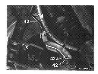
6 Remove track rod from steering knuckle arm.
