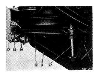
5 Separate brake line and brake hose from each other. Close connections with rubber plugs.
