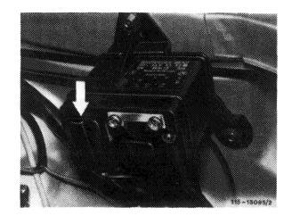
Measure resistance against ground (engine block) by means of ohmmeter one after the other at
