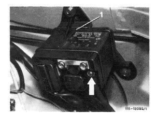
If voltage is indicated, check 80-amps fuse for tight seat or for interruption, replace fuse.
