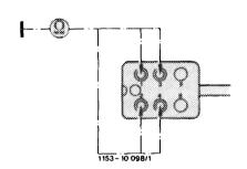
If resistance ∞ is measured, an interruption of respective pencil element glow plug or supply line or connection is indicated.
