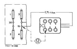
If voltage is indicated, connect voltmeter to jack 2 (terminal 15) and jack 4 (terminal 31) and test voltage.
