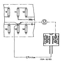
If voltage is indicated, connect voltmeter to jack 1 (terminal 15) and jack 4 (terminal 31) and test voltage.
