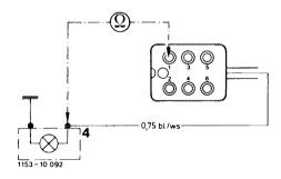
If preglow indicator lamp lights up, test green line from 8-point coupler jack 8 of preglow time relay to temperature sensor for interruption, remove interruption.
