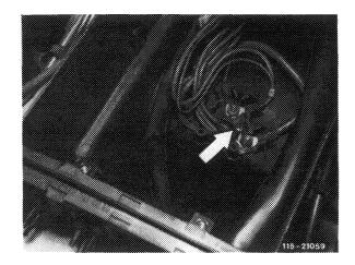
On model 123 from cable connector engine harness terminal 30 to preglow time relay connection terminal 30.
