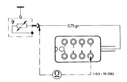
Resistance values of temperature sensor at coolant temperature:
