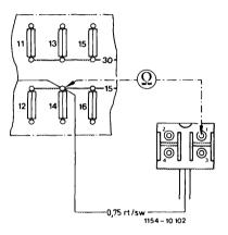
On model 123 from input fuse No. 12 to plug jack 1 of preglow time relay.
