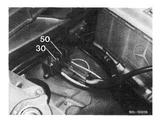
If no fault has been found up to now, test voltage on jack 1 of 4-point plug of preglow time relay against ground.
