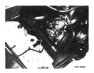
5 Unscrew water pump and remove.
