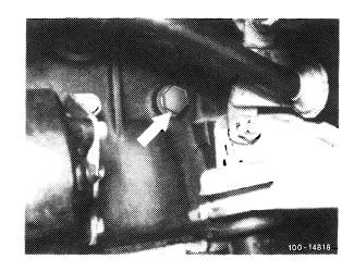
Drain plug on cylinder crankcase
