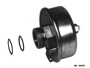
3 Mount new altitude adjusting box with washers. The venting pipe should be at the lowest point so that condensate, if any, can flow out.
