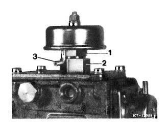
2 Unscrew altitude adjusting box. Use any washers remaining from removed altitude adjusting box, if required.
