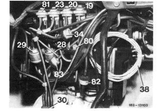
3 Pull off electrical plug and unscrew switchover valve from holder on air conditioner cabinet.
