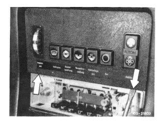
5 Unscrew both screws left and right top (arrow).
