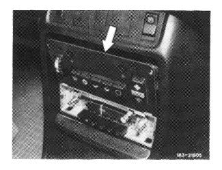
8 Unscrew three screws (arrow) and remove control unit.
