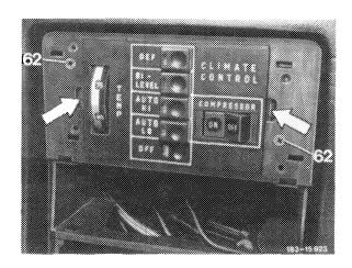
6 Pull electrical plug from optional switches and "ON/OFF" switch of refrigerant compressor (3) and remove switches.
