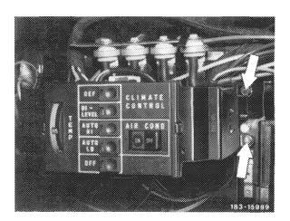
9 Pull electrical and vacuum plug connection, as well as lamps for lighting instruments from holder.
