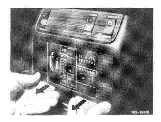
5 Remove control panel by pushing away holding pins (arrow).
