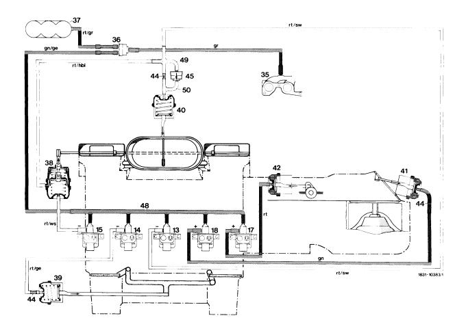
Vacuum function diagram automatic climate control Function selection "a" (defrosting)
