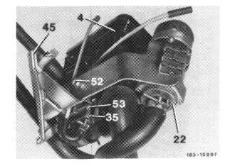
If a leak or functional trouble is suspected in entire vacuum unit, proceed according to 83-615 and perform each time the first test step (total test) of an individual vacuum circuit until the faulty vacuum circuit is found. Then continue testing the respective circuit until the fault is found.
