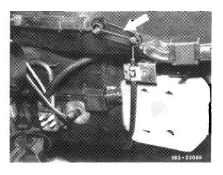
Automatic climate control Evaporator housing made by Siemens/thermal: Lever for main air flap black (arrow).
