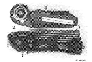
5 Take off evaporator housing lower half (3) and remove evaporator.
