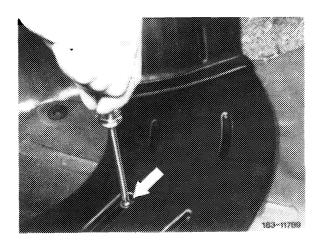
8 Remove air ducts on transmission tunnel.
