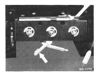
11 Force bowden wire (3) from lever of main air flap and loosen clamp (f).
