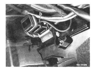
10 Separate bowden wires between operating unit on heater box and water valve.
