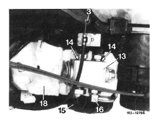
14 Pull vacuum line (26-medium green/yellow) and electric plug from temperature vacuum switch.
