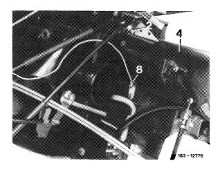
22 Remove evaporator housing from heater box, by removing nuts (2) and clamps (b).
