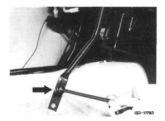
13 Unscrew refrigerant line (15 and 16) from injection valve. Then close with plug.
