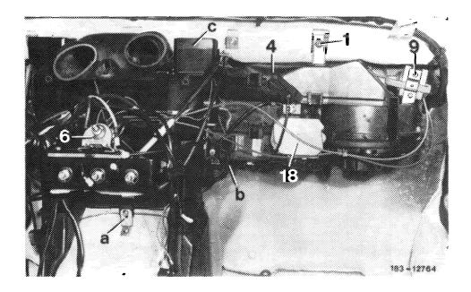
16 Unscrew nut (1) and angular fastening bracket (a).
