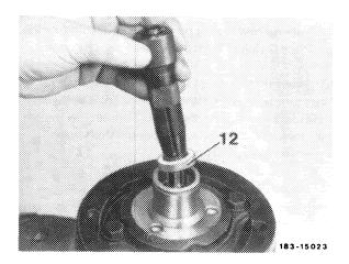
6 Remove shaft sealing (13) by means of disassembling and assembling tool. For this purpose press on tool, then turn tool to the right in order to grip projection on shaft sealing by means of the locking tongues on the tool. Completely remove shaft sealing from shaft by pulling in straight-forward direction.
