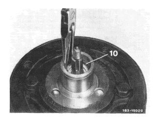
5 Remove slip ring (12) by means of disassembling and assembling tool.
