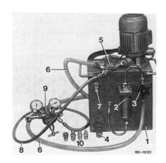
The R 11 cleaner can be used several times. As soon as the cleaner looks rather cloudy (showing up when flowing through PVC hoses (6), renew together with KC dry pearls in filter drier (2).
