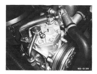
2 Screw line connection reduction piece (26) on supply bottle (16). Connect filling hose (5) to reduction piece (26) and blow through for a short moment with refrigerant to remove remains of dirt and moisture, if any, then connect filling hose (5) to connection (6) (suction side) of service valve (offset end with pressure pin of hose line).
