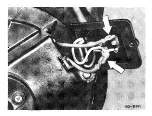
5 Remove screws from blower motor flange.
