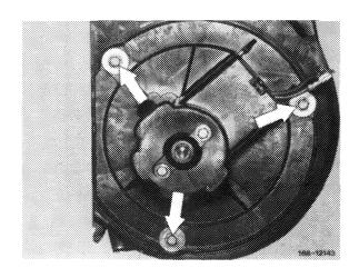
6 Lift blower motor out of blower housing.
