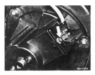
4 Lift contact plate and pull off both connecting wires for series resistance.
