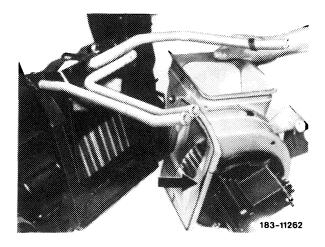
11 Lift heat exchanger in upward direction out of heater box.
