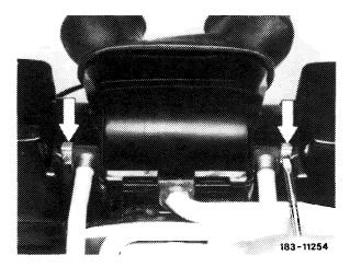
4 Remove both clamps on front end of cover.
