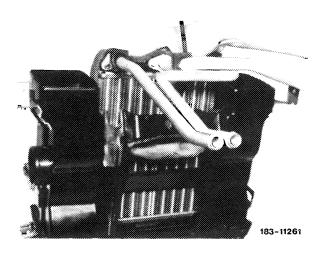
12 Remove seals from water pipes.
