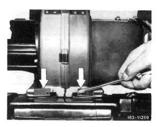
9 Remove both rubber seals from water pipes.
