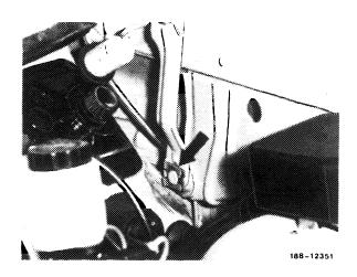
6 Remove both screws from engine hood.
