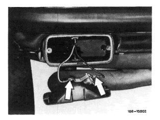
3 Unscrew fastening nut on bumper bracket left and right and pull out bumper toward the rear.
