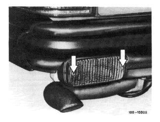
2 Pull reflector on back-up lamp and on fog lamp from lamp housing and pull off the two cables.
