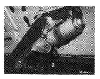
7 Remove complete system from rear holder (4) and pull off coupler for electric connections (3). Completely remove wiper system.
