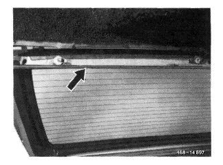
5 Unscrew fastening screws (1) of wiper system.
