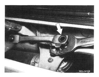
6 Remove water drain from righthand bearing shaft.
