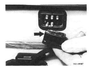
8 Unclip plug from direction of fresh air chamber (arrow) and pull through front wall.
