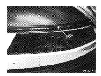
4 Remove cover (1), center. Remove 4 expanding rivets (2). Remove one Phillips head screw (3) each at left and right of cover.
