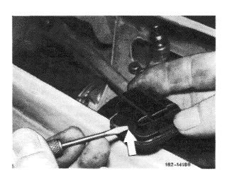
9 Remove fastening screws (1) of wiper motor.
