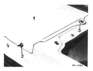
5 Pull connecting rod left and right from wiper motor crank.
