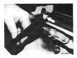
7 Pull off coupler (accessible from engine compartment).
