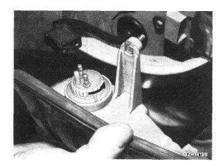
3 Remove bulb out of socket by means of a light lefthand turn (bayonet lock).
