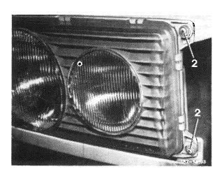
5 Disconnect guide lug of lamp unit on fender.
