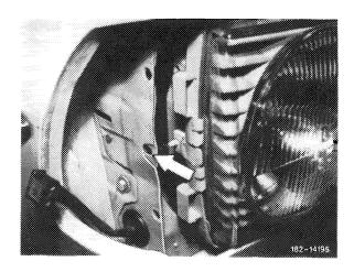
6 Pull off coupler for electric connections and remove lamp unit.
