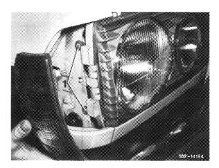
4 Unscrew fastening screws (2) inside on lamp unit.
