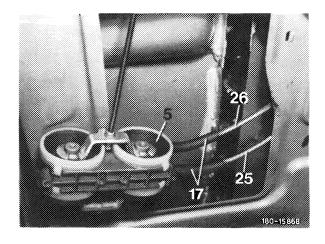
6 Pull off lock washer (43) of control rod (2) on vacuum element (5) and pull out control rod.
