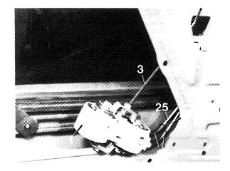
8 Pull lock washer (43) of control rod (3) from vacuum element (1) and pull out control rod.
