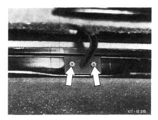
7 Unscrew rear roof frame clamp.
