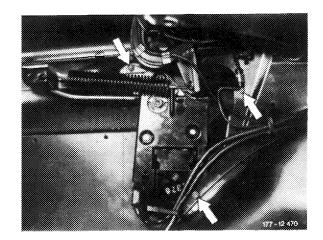
6 Unscrew mounting bolts of retaining plate for teleflex tube on sun roof frame.
