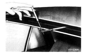
5 If the teleflex cable cannot be removed even after dismantling the gearbox, the teleflex tube has been damaged and must be removed (77–150).
