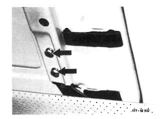
Note: Since the sun roof frame will have tolerances in the overall width, it will be necessary to check the side clearance at several points. Always make sure that the sun roof lid opens and closes correctly.
