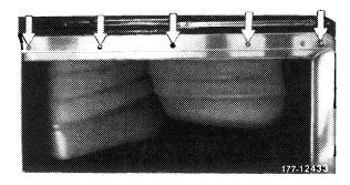
3 Shut sun roof lid and remove left and right lock screws.
