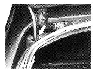
4 Unscrew front fastening screw (hex. socket) through assembly hole in head lining.
