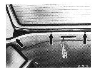
3 Pull out safety clip on rear fastening of gas pressure spring and push out bolt in outward direction.
