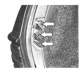
8 If back door binds in lock, adjust by removing or inserting a spacing washer at lock strap to adjust distance in relation to lock.
