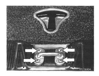
9 Adjust lateral distance of back door by adding shims to stop on back door (left or right).
