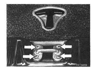
7 Tighten screws on stop of rear pillar and on strap for back door lock.
