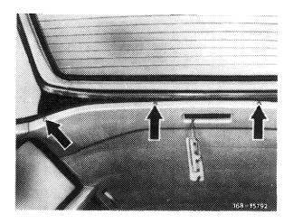
2 Loosen cable connections on roof frame and disconnect cable harness from holding clips on roof frame.
