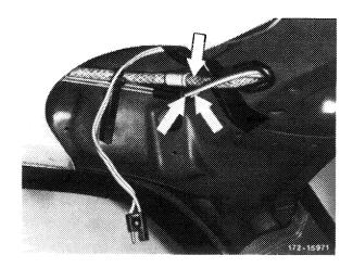
13 Connect electric lines from the left to the right (in driving direction).
