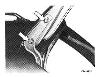
11 Attach gas pressure spring to hinge and secure.
