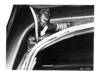
12 Connect water hose for back window washer (with central locking system also the vacuum lines).
