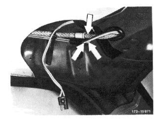
6 Pull out safety clips from rear attachment of gas pressure switch and push out bolts in outward direction.
