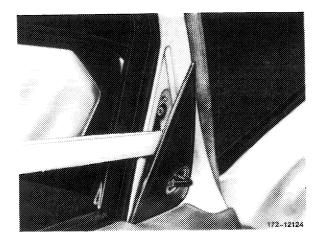
4 Unscrew screws and remove mirror.
