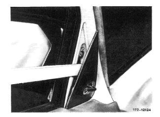
4 Unscrew screws and remove mirror.
