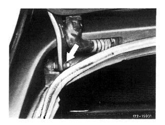
12 Connect water hose for back window washer (with central locking system also the vacuum lines).
