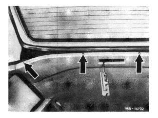
2 Loosen cable connections on roof frame and disconnect cable harness from holding clips on roof frame.
