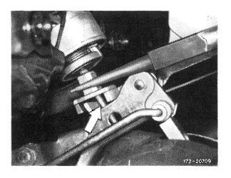
Note: Insert trigger foot in such a manner that the chamfered driving lug is below.
