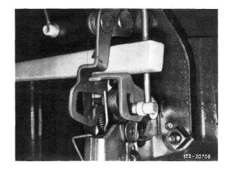
4 Insert screwdriver through bore for upper lock attachment and turn adjusting screw for relief clearance to the right until trigger foot slides out of snap lock onto screwdriver.
