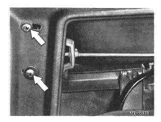
13 Latch the lock by means of safety plunger. Adjust relief clearance (1 mm) by inserting a small screwdriver through the thread of the upper lock attachment. Install upper securing screw in back door lock.
