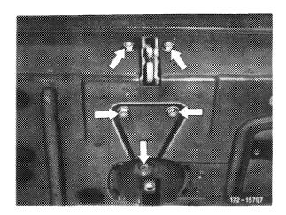
10 Attach plug for back door contact switch to right-hand side of lock.
