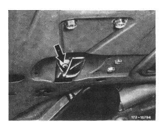
4 Pull plug for back door contact switch from right-hand side of lock.
