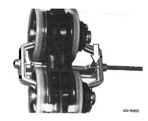
6 Unscrew fastening screws of door lock.
