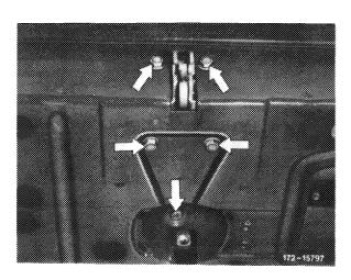
7 Lock rotary catch of lock. This will make the lock less wide for easier removal.
