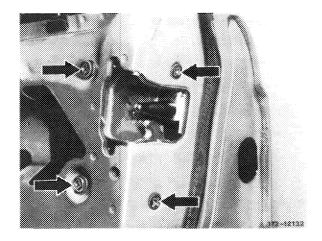
5 Remove door lock with cover from door downward.
