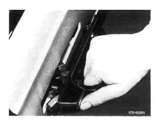
6 Press back door grip, making sure that drive screw engages in door lock. If pre-load between outside door panel and front mounting screw is not sufficient, adjust screw accordingly.
