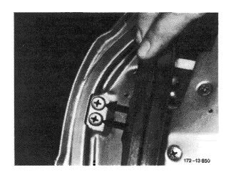
6 On door handle with safety lock, insert ignition key into lock cylinder. Turn ignition key approx. 50° to the rear and remove door handle.
