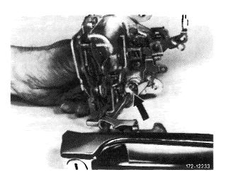
9 On door handle with safety lock, pull grip and insert handle in door cutout. Simultaneously turn lock cylinder with ignition key 50° to the rear and introduce turning rod into turning nut on lock.
