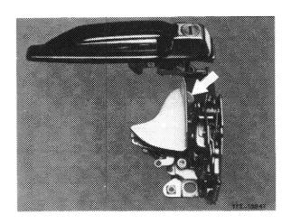
10 On door handle with safety lock, pull grip and insert door handle into cutout of door. Simultaneously turn lock cylinder approx.  $50^{\circ}$  to the rear by means of ignition key and introduce turning rod into turning nut on lock.
