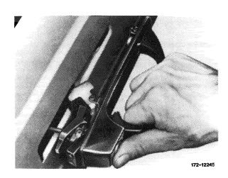
8 Guide rotary rod into rotary nut.
