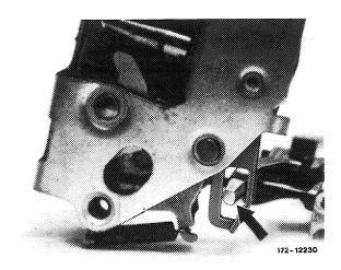
**Note:** The clearance between the drive pin and opening on the door lock should be about 1 mm. Adjustments are made with the socket screw.
