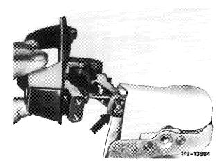
**Note:** Play between driving pin and cutout at door lock should be approximately 1 mm. Adjustment is made with the hexagon socket screw.
